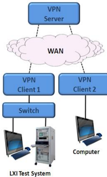
Figure 3.6 Configuration Using VPN Connections
